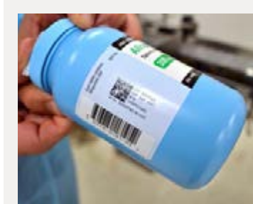
Serialization ensures that medicines can be tracked and traced through the supply chain.
